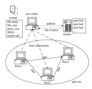
Fig. 2. BitTorrent deployment scenario
