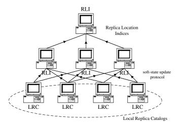
Fig. 1. Replica Location Service deployment scenario
