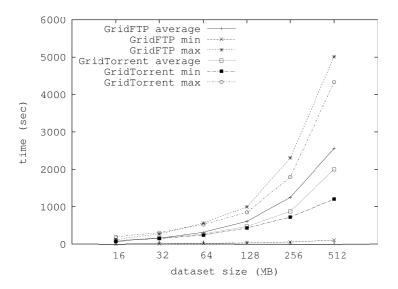
Fig. 4. Minimum, maximum and average time required for 16 independent downloaders to transfer a file using either GridFTP or GridTorrent
