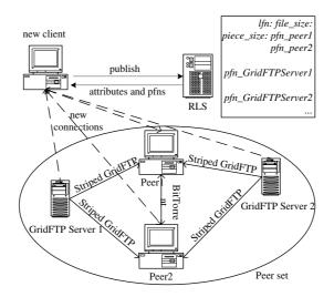
Fig. 3. GridTorrent deployment scenario
