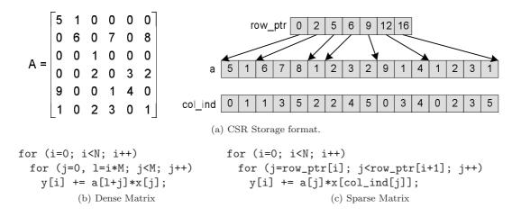
Figure 1: Example of the CSR storage format, dense and sparse matrix-vector multiplication kernels.
