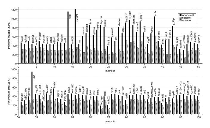
Figure 4: Performance of the SpMxV kernel: MFLOPS for each matrix and architecture.
