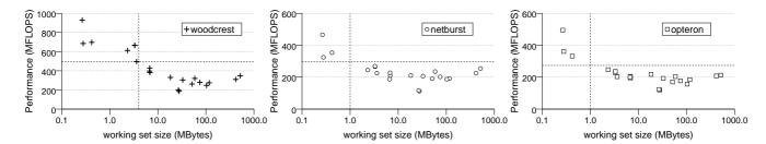
Figure 7: Performance of matrices with small number of elements, less than 8 for 80% or more of their rows, in relation to their working set. Vertical line marks the L2 cache size for each processor. Horizontal line marks the average performance.
