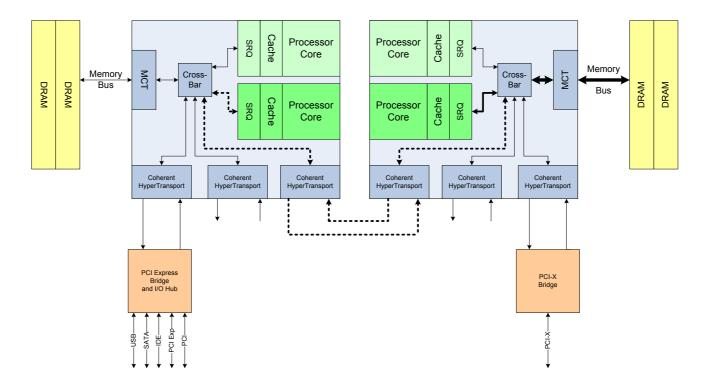
Figure 17: Contention of main memory requests on *Opteron*. All data are stored on a single memory node (right bank). As a result, one core needs to perform remote memory accesses (dashed line), which eventually lead to contention on the common memory controller and memory bus (bold line).
