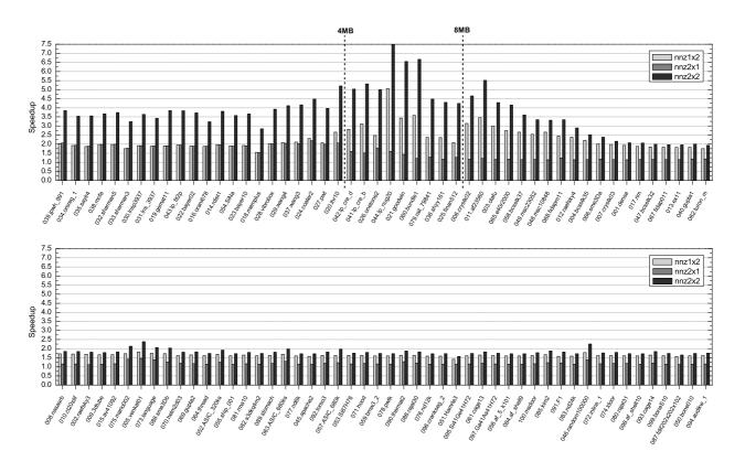
Figure 12: Speedup achieved on *Woodcrest* for every multithreading scheme. The first vertical line denotes the effective cache size for the serial execution and the  $1 \times 2$  multithreading scheme, and the second one denotes the effective cache size for the  $2 \times 1$  and  $2 \times 2$  multithreading schemes.
