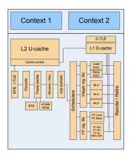
Figure 2: The HyperThreading technology of the *Netburst* microarchitecture. The architectural state of the processor is duplicated, thus forming two logical processors recognized by the operating system. Every other resource of the processor is dynamically or statically shared between the two hardware contexts.
