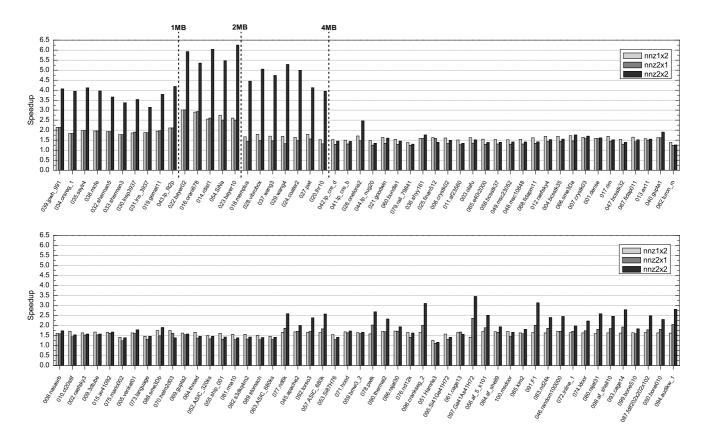
Figure 13: Speedup achieved on *Opteron* for every multithreading scheme. The vertical lines denote the effective cache size for the serial execution, the  $1 \times 2$ ,  $2 \times 1$ , and  $2 \times 2$  multithreading schemes, respectively.
