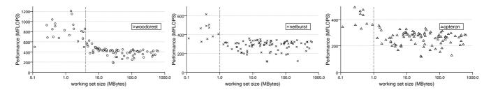
Figure 5: Performance of the SpMxV kernel in relation to the working set size for all architectures. The vertical line in each graph designates the size of the L2 cache for each architecture.
