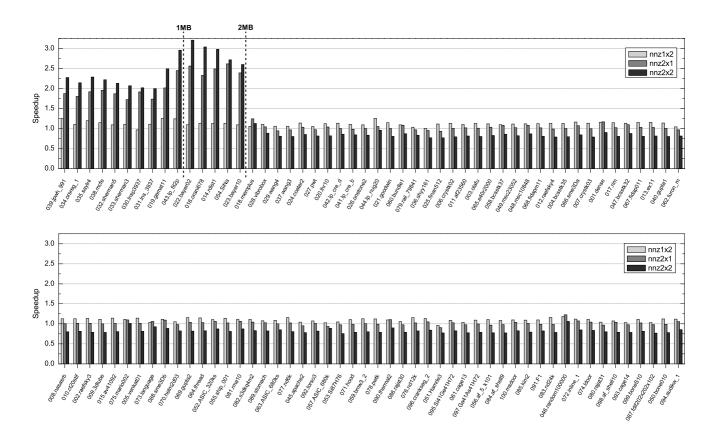
Figure 11: Speedup achieved on *Netburst* for every multithreading scheme. The first vertical line denotes the effective cache size for the serial execution and the  $1 \times 2$  multithreading scheme, and the second one denotes the effective cache size for the  $2 \times 1$  and  $2 \times 2$  multithreading schemes.
