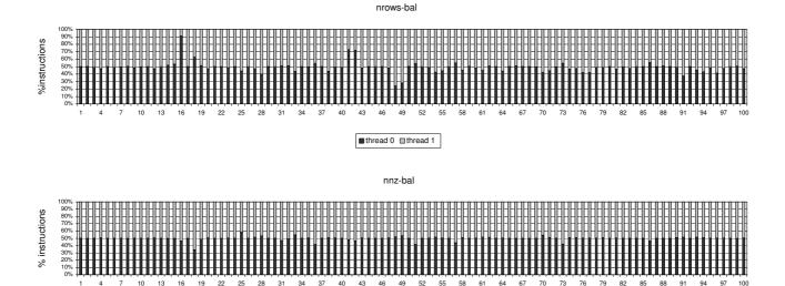
Figure 10: Load distribution (total instructions executed) between the row-based and the non-zero-based partitioning schemes. The non-zero-based scheme leads to much better load distribution.
