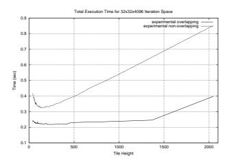
Figure 7. MPI over TCP/IP over FastEthernet: Results for 32x32x4096 space
