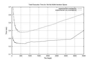
Figure 5. MPI over TCP/IP over FastEthernet: Results for 16x16x16384 space
