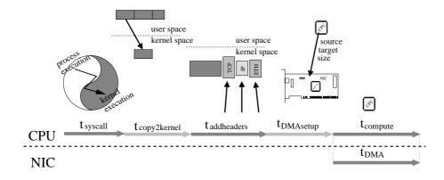
Figure 3. Successive sending phases for a packet, including CPU and NIC. (a) CPU execution switches from user to kernel mode, (b) CPU copies data from user space to kernel space, (c) CPU adds protocol headers, (d) CPU sets up DMA engine, (e) NIC DMA transfers data to its buffers, while CPU is free for computations
