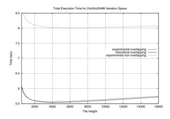
Figure 14. Experimental Total Execution Times for  $24 \times 24 \times 2048K$
