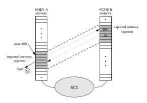
Figure 8. SCI load/store instruction over exported segment: (a) process on node A writes value 100 to a location in the imported segment and the value is transferred to node B exported segment, (b) process on node A reads a location in the imported segment and the value 50 is transferred from node B exported segment
