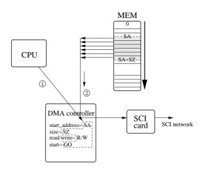
Figure 9. DMA or nonblocking send
