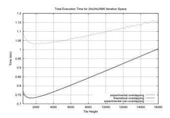
Figure 13. Experimental Total Execution Times for  $24 \times 24 \times 256K$
