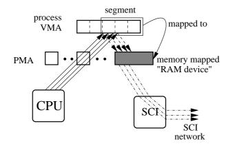
Figure 10. Locked (pinned down) and memory mapped "RAM device" for SCI communications. While CPU computes data, results are stored to physically contiguous memory, ready to be sent as a whole using DMA
